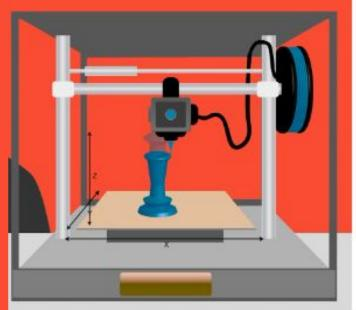
First melted plastic goes through a small tube. Then goes into a valve then layer by layer add More and more layers like icing on a cake.
